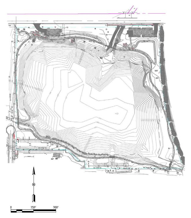
Figure 1-3. Bathymetric Contour Map for Booker Lake. (Elevations based on City of St. Petersburg datum).
