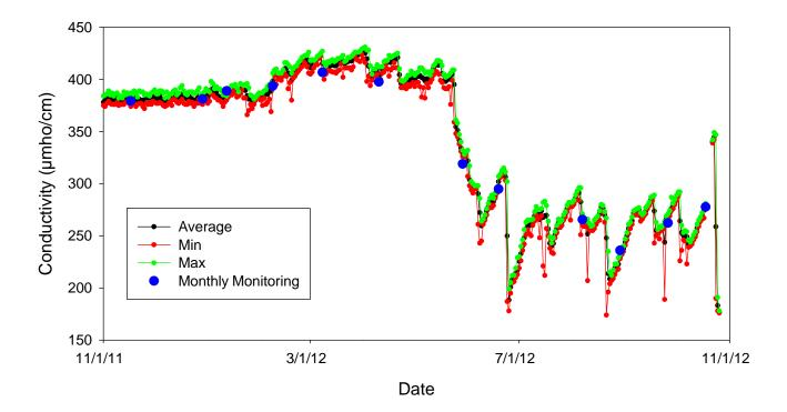
Figure 4-7. Continuous Field Measurements of Conductivity in Booker Lake Collected by the YSI Datasonde from November 2011-October 2012.
